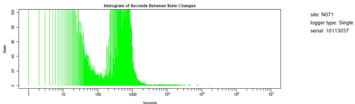
Navigant generated weekly, monthly, and seasonal graphs to ensure the blower motor operation, gas valve operation, and indoor temperature data were consistent. Figure 4-3 shows an example of these weekly graphs, which in this particular case Navigant determined the dataset to be reasonable based on
