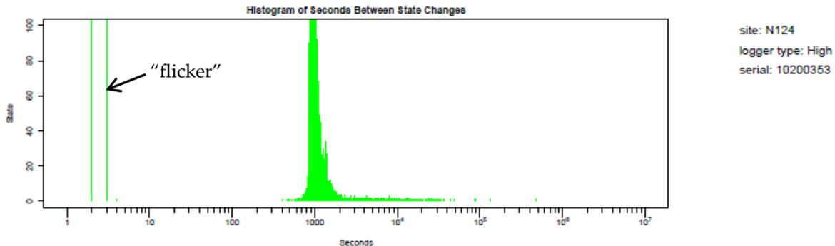
The x-axis is a logarithmic scale of event duration, and the y-axis shows the frequency of event durations. The two spikes and two and three seconds likely indicate flicker (due to nearby currents or startup pulses) and not actual gas consumption.
